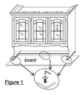
One board was secured to the bottom of Hutch with three bolts and three flat washers for the shipping safety purpose only. Please disassemble the board by using the Allen key and throw away the board. (Figure 1.)
